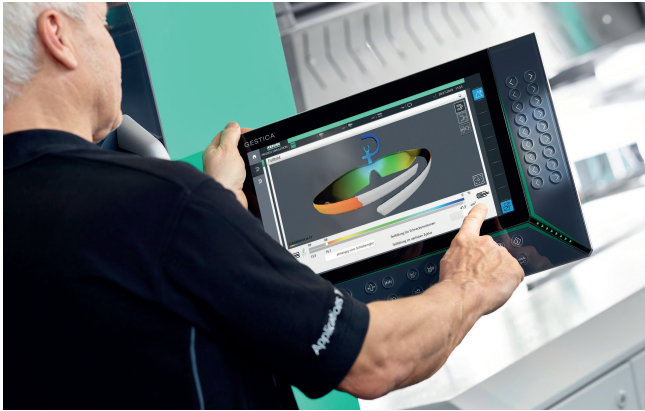
Fig. 5. The "aXw Control FillAssist" shows the operator what is currently taking place in the mold © Arburg
